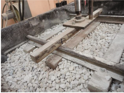
Fig. 10. Lowering the load spreader beam to touch the track.
